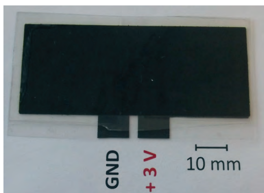
Figure 4: A 3V_{nom} battery (left) and its discharge curve at 1 mA (right). (Willert et al., 2013a)
