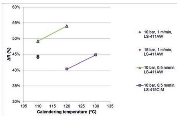
Figure 5: Antenna resistance changes ( $\Delta R(\%) = (R_{\text{initial}} - R_{\text{calendered}}) / R_{\text{initial}}$ ) of printed Asabi LS-411AW and LS-415C-M sheets during R2R calendering using different calendering temperatures, speeds, and pressures
