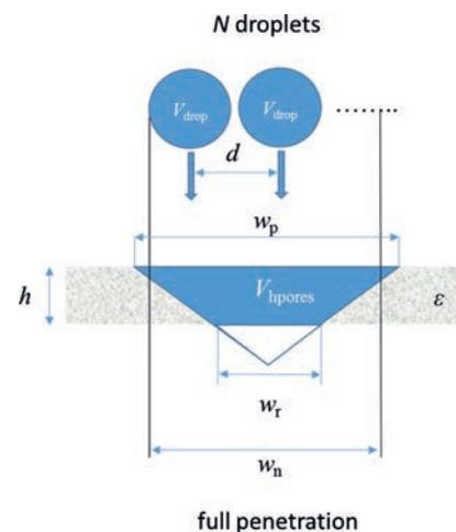
Figure 9: Schematic showing the applied drop volume  $V_{\text{drop}}$  with a drop spacing  $d$ , which is applied to the substrate of thickness  $h$  to form a nominal transverse barrier width  $w_n$ , having a wedge-shaped cross-section of width  $w_p$  and  $w_r$  on the printed and reverse sides, respectively, such that the pore volume affected by the hydrophobising agent is  $V_{\text{hpores}}$
