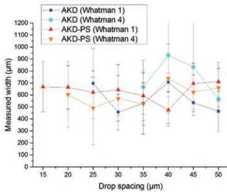
Figure 7: Measured widths of reliable barriers printed with AKD and AKD-PS inks
