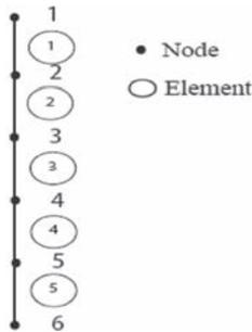
Figure 3: 1-D element model system of Figure 1
