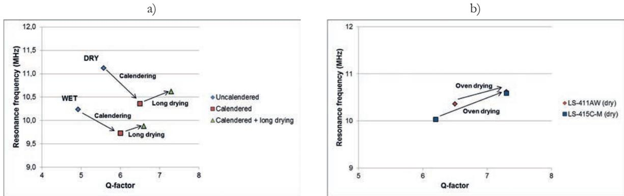
Figure 11: a) Resonance frequencies and Q-factors of the moisture sensors as a function of calendering, long oven drying, and moisture content; under wet environment, the resonance frequencies and Q-factors are lower; b) Effect of the ink type on the Q-factor of the printed moisture sensors; the LC-circuit layer was calendered in R2R process
