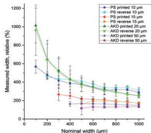
Figure 4: Relative line widths, in terms of nominal width, for Whatman 4 filter paper printed with PS ink at 10 and 15  $\mu\text{m}$  drop spacing, and with AKD ink at 20 and 50  $\mu\text{m}$  drop spacing
