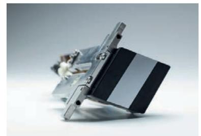
FUJIFILM Dimatix, Inc. places extra emphasis on dot placement accuracy, channel-to-channel uniformity, low cross talk and high frequency/high productivity. The new Samba drop-on-demand inkjet printheads have 2,048 individually addressable nozzles, delivering 1200 dpi native resolution
