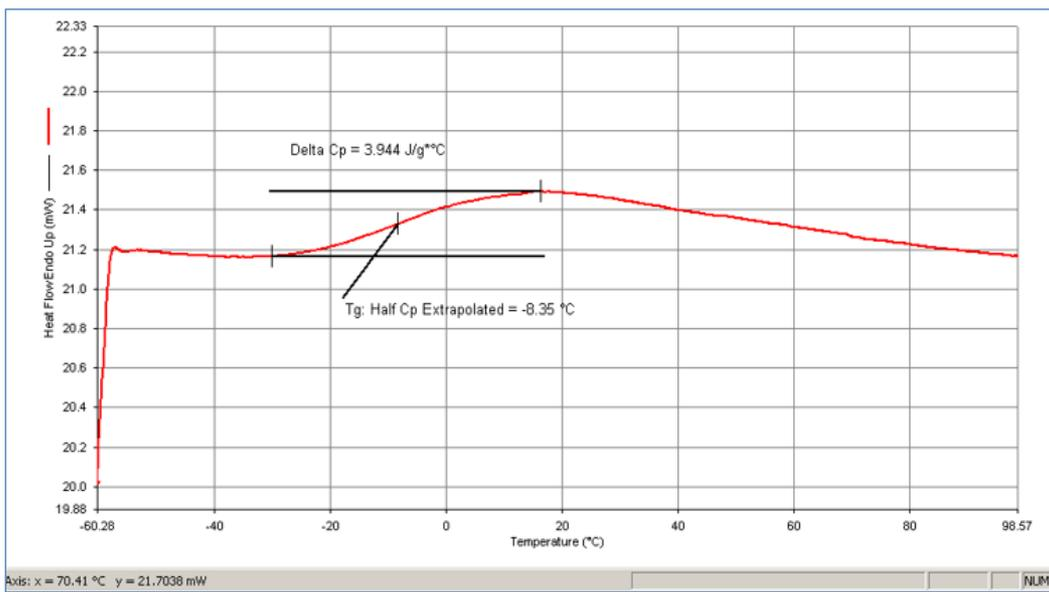
Figure 3: The DSC curve of PUD at 1.4 NCO:OH ratio
