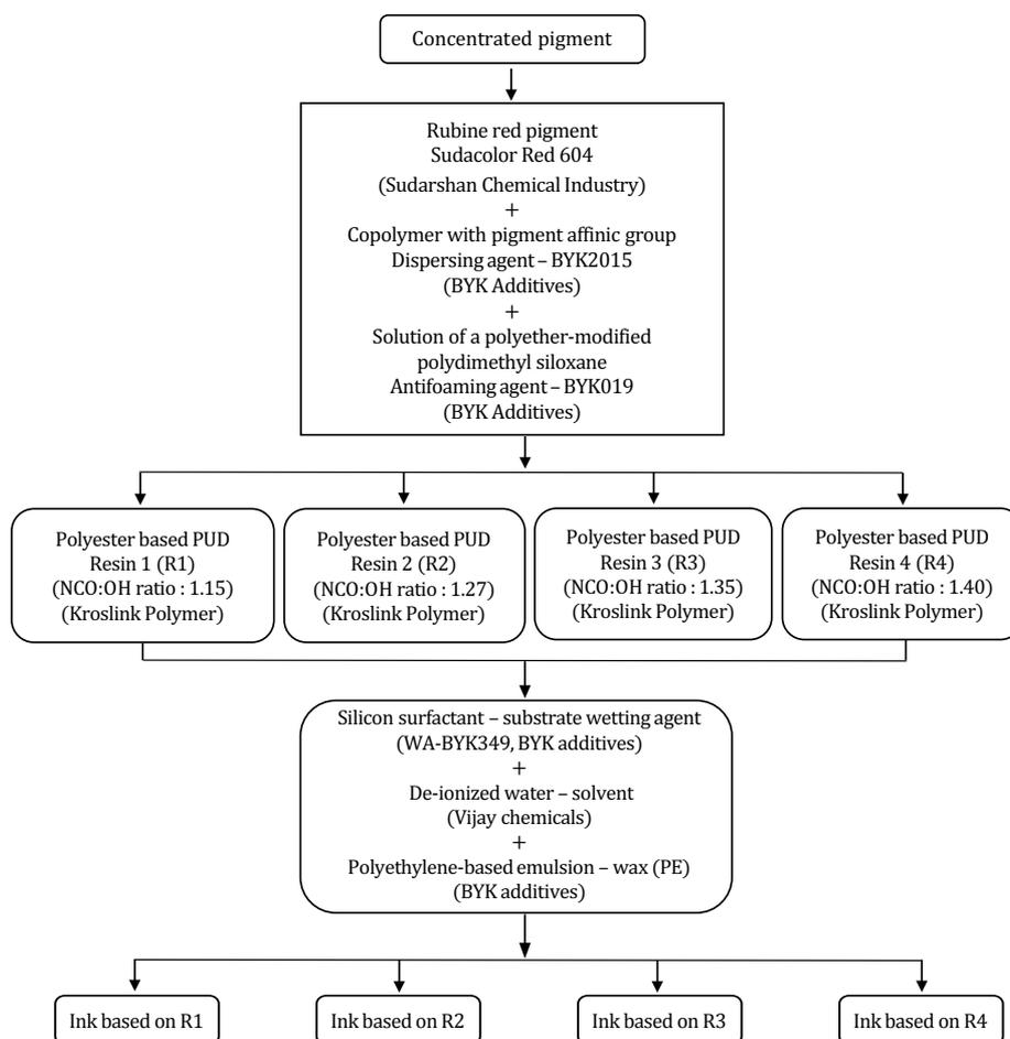
Figure 1: Flowchart for ink ingredients and stepwise addition
