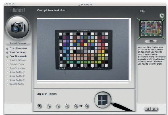
Figure 3: X-rite Eye-One Match 3 application with a photo of a ColorChecker Digital SG test chart
