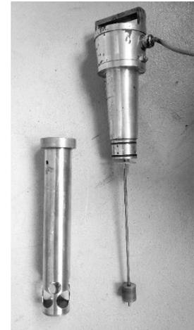
Figure 2: Rotary viscometer with cylindrical test block
