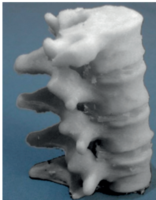
Figure 5: 3D printed bone vertebra structure
