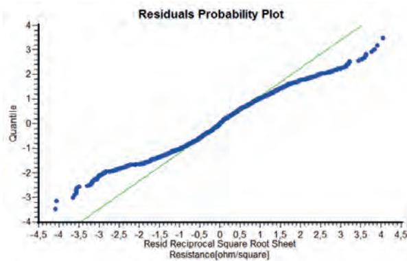
Figure 12: Residuals Probability Plot for distribution of the measured and then transformed sheet resistance values of printed cold foil samples
