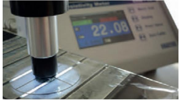
Figure 8: The contactless sheet resistance measurement system SRM-14TSS of company NAGY Messsysteme GmbH (NAGY, 2014)
