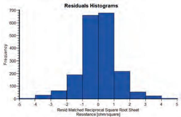
Figure 11: Residuals Histogram for distribution of the measured sheet resistance values of printed cold foil samples
