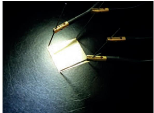
Figure 7: Sheet resistance measurement of a printed cold foil sample on the 4-point measurement station
