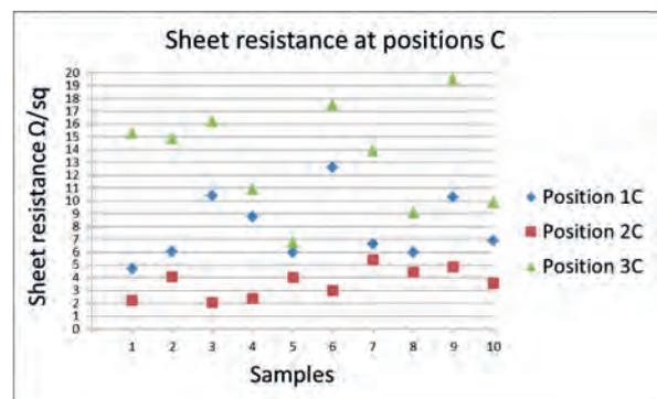
Figure 9: Sheet resistance values of cold foil samples for test run number 14 at positions A, B and C (Type 1 cold foil material); for the positions 1A to 3C see Figure 5 and Figure 6
