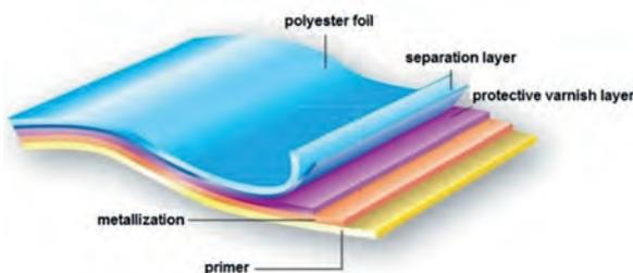
Figure 1: The layer composition of a cold foil (Kurç, 2011)
