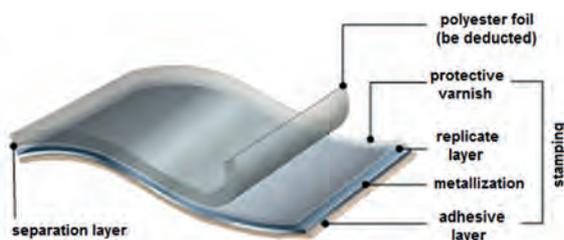
Figure 2: The layer composition of a hot stamping foil (Kurç, 2011)
