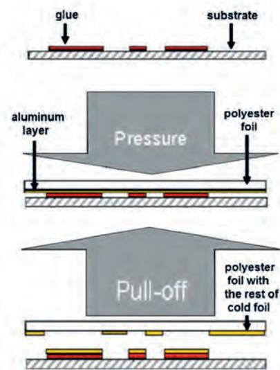
Figure 3: Working principle of cold foil transfer process (Heidelberg, 2012)
