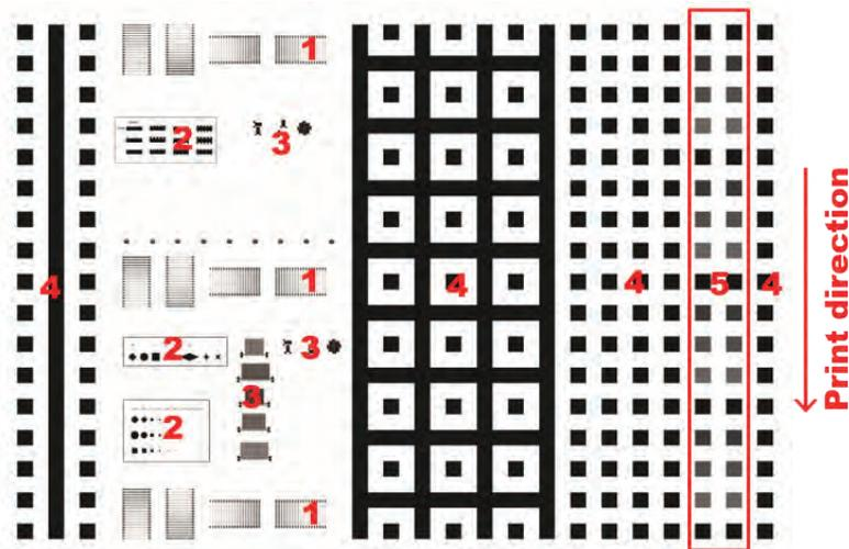
Figure 4: Sheet layout in format  $1050 \times 750$  mm for printing experiments: 1 – circuit paths; 2 – visual control elements; 3 – sensor elements; 4 – full tone fields; 5 – half tone fields (10–100 %); print direction shows direction of sheet running in the offset printing press, in other words, the leading edge of the print sheet is shown in the lower edge of the image
