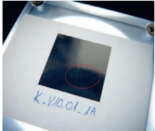
Figure 13: A printed cold foil sample on the illuminated field of the NAGY system SRM-14TSS with a marked position of a crack in the metal layer
