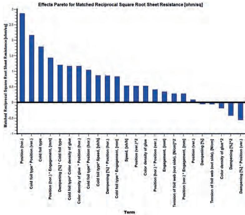
Figure 10: Chart Effects Pareto for the influence of input variables (printing setting) on the examined output variable (electrical sheet resistance of printed cold foil samples)
