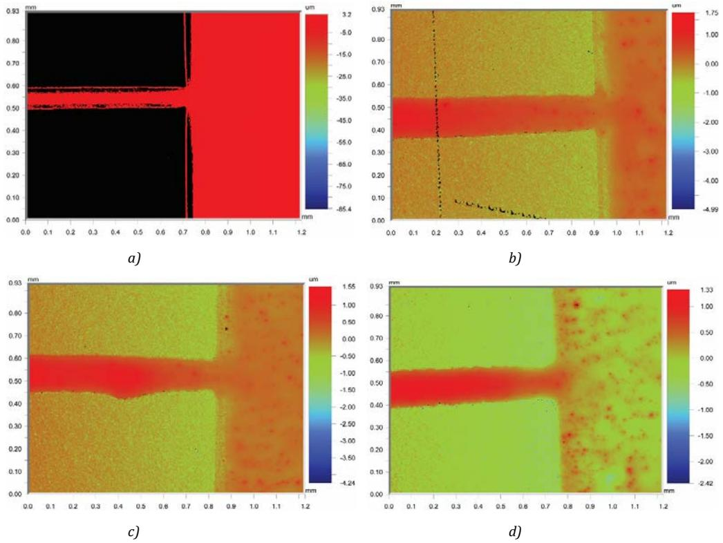
Figure 7.3: 100-μm line and pad joint on: a) printing plate, b) print without UV-ozone treatment of plate, c) print obtained by plate UV-ozoned for 2 minutes, d) print obtained by plate UV-ozoned for 5 minutes
