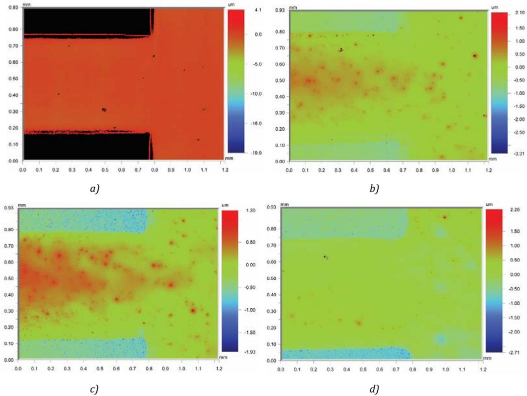
Figure 7.4: 600-μm line and pad joint on: a) printing plate, b) print without UV-ozone treatment of plate, c) print obtained by plate UV-ozoned for 2 minutes, d) print obtained by plate UV-ozoned for 5 minutes
