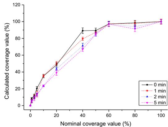
Figure 9: Coverage values of halftones on prints produced by UV-ozone treated plates
