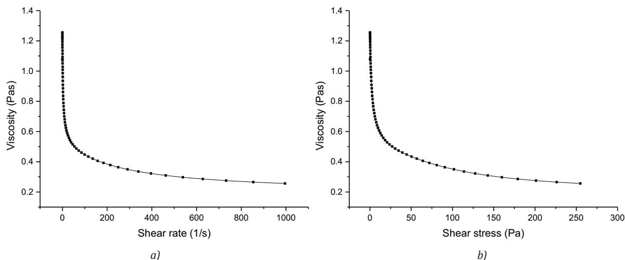
Figure 2: a) Viscosity vs. shear rate of the printing ink, b) viscosity vs. shear stress of the printing ink
