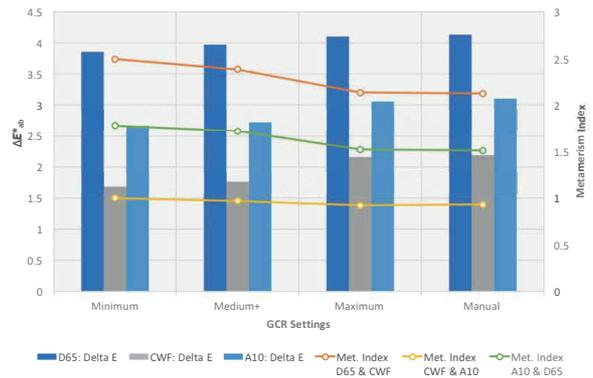
Figure 9: The  $\Delta E^*_{ab}$  &  $MI$  of Galaxy Oak patch with 7 g/m<sup>2</sup> release coat plus tie coat
