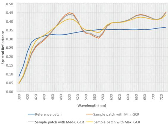
Figure 12: Spectral curve of Smooth Grey patch with 7 g/m<sup>2</sup> release coat with different GCR settings
