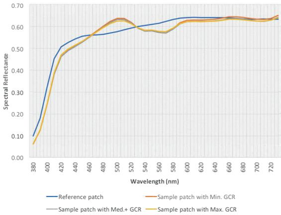
Figure 11: Spectral curve of Galaxy Oak patch with 7 g/m<sup>2</sup> release coat with different GCR settings
