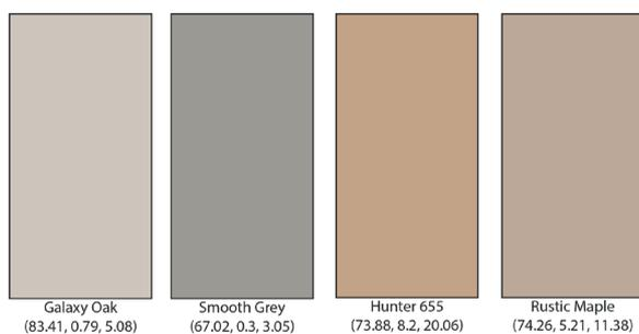
Figure 1: Sample patches, with CIELAB values
