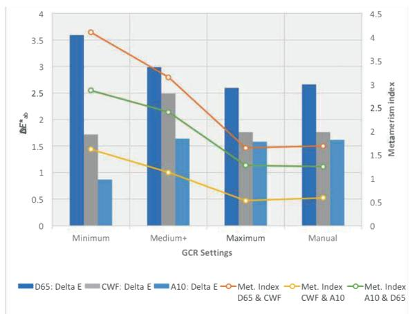
Figure 10: The  $\Delta E^*_{ab}$  &  $MI$  of Smooth Grey patch with 7 g/m<sup>2</sup> release coat plus tie coat
